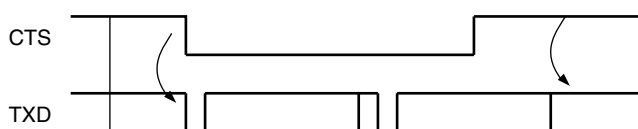
Figure 33-17. Transmitter Behavior when Operating with Hardware Handshaking
